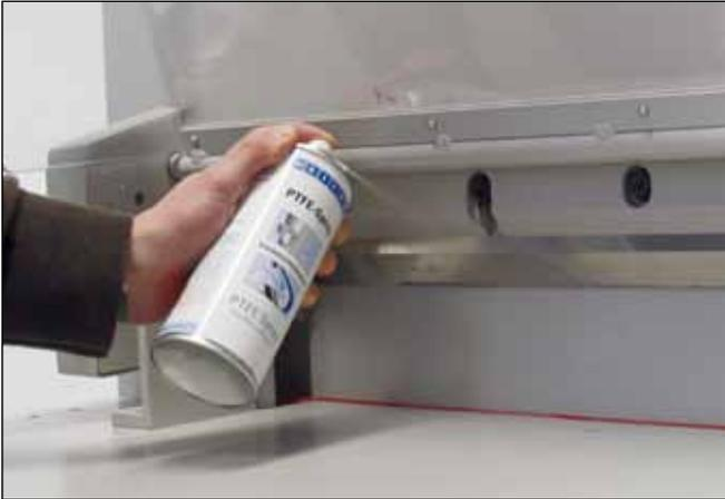
WEICON PTFE-Spray adheres to all metal, plastic and wood surfaces. Due to the high PTFE percentage, the coefficient of friction is considerably reduced. The coating is resistant to dirt, dust, water, oils, greases, and many chemicals. Temperature resistant from  $-180^{\circ}\text{C}$  ( $-292^{\circ}\text{F}$ ) to  $+250^{\circ}\text{C}$  ( $+482^{\circ}\text{F}$ )
