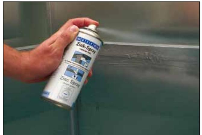
WEICON Zinc Sprays are dust-dry after about 15 minutes and can be spackled and painted over after about 12 hours without pretreatment. The temperature resistance amounts to up to  $+500^{\circ}\text{C}$  ( $+932^{\circ}\text{F}$ ) (in the case of "bright grade", up to  $+300^{\circ}\text{C}$  /  $+572^{\circ}\text{F}$ ).
