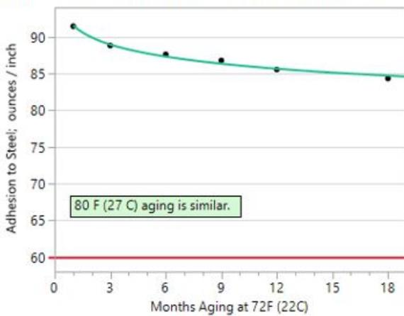
Adhesion to Steel (72F (22C)) of tape Conditioned to Varied %RH
