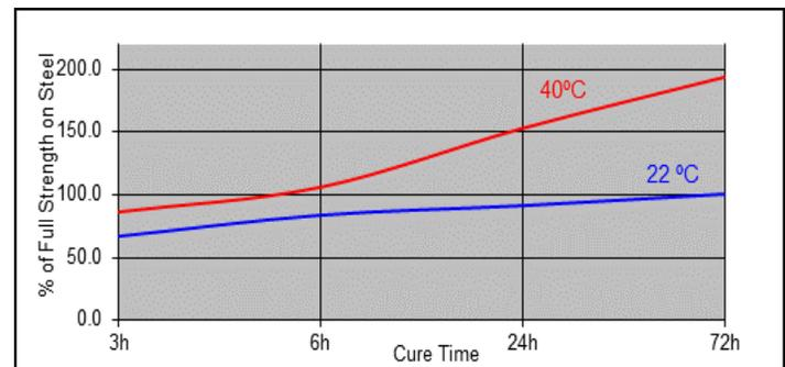
The table below shows breakloose torque developed with time on 3/8inch NPT steel pipe tees and plugs, pre-torqued to 238 in-lb and tested according to ASTM D6396.
